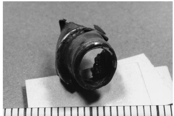
Fig. 1 Projectile fragment, erroneously considered to be the jacket of a larger-caliber bullet beside the head of the victim
