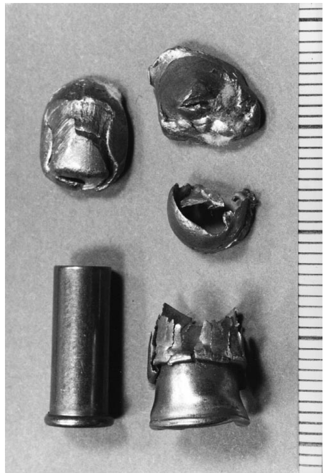
Fig. 3 Deformations of the tandem loaded projectiles (.22lr Remington ammunition); left: parts of the normally loaded projectile, right: parts of the muzzle-loaded projectile
